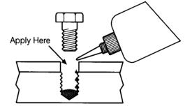
7. Assemble and tighten as usual. When tightening to established torque values, torque compensation is not required.
