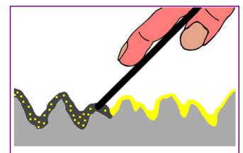
Immediately afterwards apply the required layer thickness on the still soft Polymer Metal:
