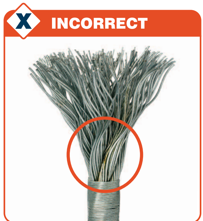
Figure 4: Incorrectly broomed wire rope.
