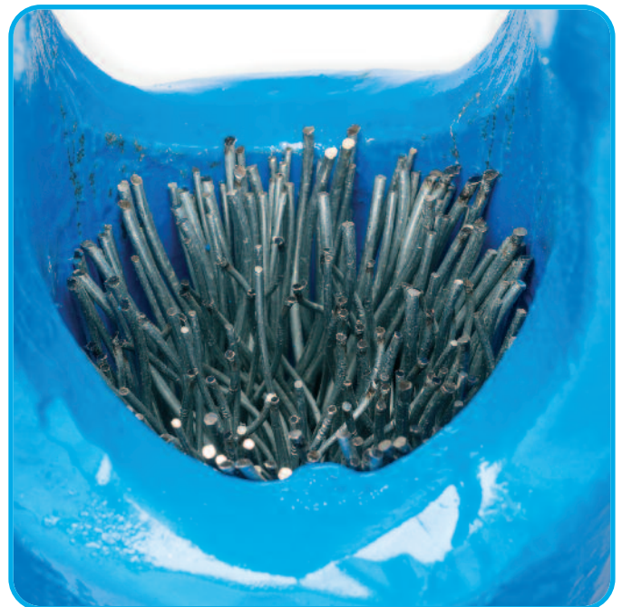
Figure 5: Properly positioned broom with the wire ends protruding slightly.
