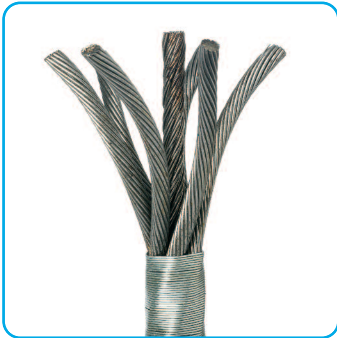
Figure 2: Unlay wire rope so that the angle does not exceed 90°.
