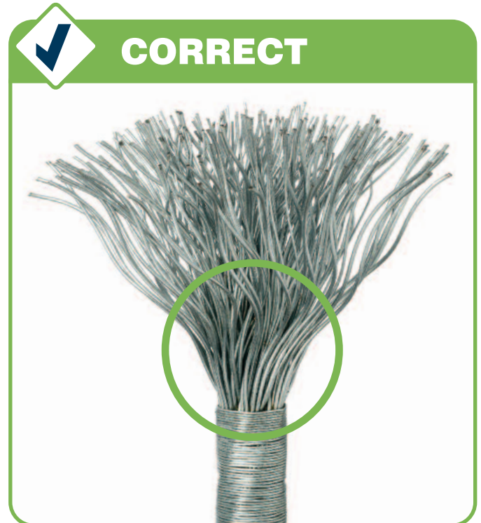
Figure 3: Properly broomed wire rope unlaidd from the end of the rope to the seizing.
